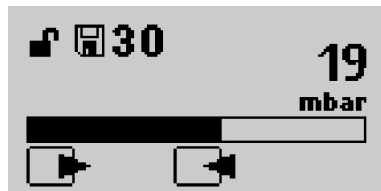
Fig. 25: Gas flushing status display (049)
