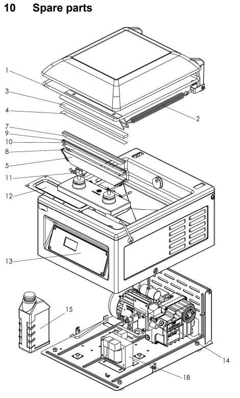
Fig. 30: Spare parts drawing
