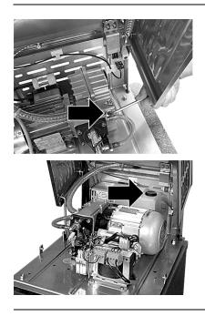
> Unscrew the screw plug of the oil fill opening.
