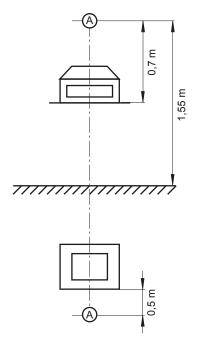
Fig. 29: Noise exposure measuring point
