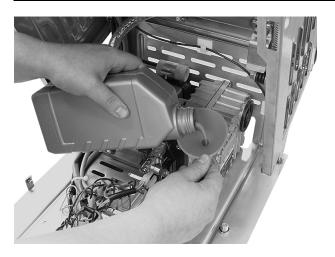
Fill the vacuum pump with oil up to the middle of the oil sight glass. Use only oils that are approved by the manufacturer, see 'Spare Parts' section or the spare parts list.
