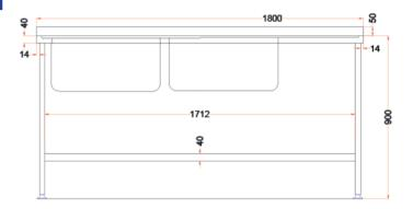
This fully welded 1800mm wide sink from Holmes features a right side drainer with double bowl on the left side, and a convenient undeshelf providing extra storage for supplies and utensils. The sink is made with 304 stainless steel, making it smooth, hygienic and easy to clean whilst offering high resistance to corrosion and staining. The sink is perfect for creating practical and hygienic washing areas in any commercial kitchen.
