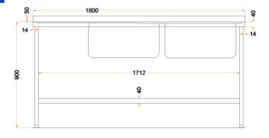
This robust, fully welded 1800mm wide sink from Holmes features a left side drainer with double bowl on the right side, ideal for creating hygienic and practical washing areas in your kitchen. The sink is constructed from 304 stainless steel, which is smooth, easy to clean and offers high resistance to corrosion and staining. It also features a strong undershelf which provides additional storage for utensils and supplies.
