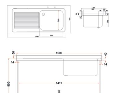
This fully welded 1500mm wide sink from Holmes features a left side drainer with right side bowl, and a strong undershelf for extra storage. The sink is made with 304 stainless steel, which is smooth and hygienic whilst offering high resistance to corrosion and staining making it perfect for use in commercial kitchens. The sink is ideal for creating practical and hygienic washing areas that are easy to keep clean.
