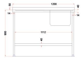
The fully welded 1200mm wide sink from Holmes is made from commercial grade stainless steel, and features a left side drainer with right side bowl. The 304 stainless steel is highly resistant to rusting and stains, as well as smooth and easy to clean which makes it ideal for use in commercial kitchens. The sink allows you to create practical and hygienic washing areas in your kitchens, and features a strong, sturdy undershelf for the additional storage of supplies and utensils.
