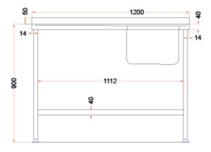
This fully welded 1200mm wide sink from Holmes features a left hand drainer with right hand bowl, and is easy to assemble. The sink is made with 304 stainless steel, which is smooth, hygienic and easy to clean whilst offering high resistance to corrosion and staining making it perfect for use in commercial kitchens. Create practical and hygienic washing areas in your kitchen with this commercial sink which also features a strong undershelf for extra storage.
