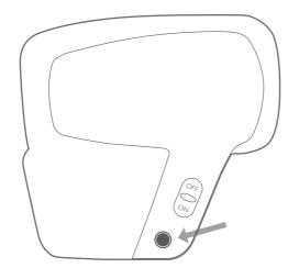
Hang the base unit on the bracket. Align the product with a spirit level and mark with a pencil through the bottom hole.
