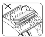
Place the banknotes in the centre of the hopper. The NC30 will start counting automatically or the "RESTART" button will need to be pressed, see "3.3 Automatic or manual start". The quantity of banknotes counted will be displayed in the counting result display. If a counterfeit or different denomination is detected the NC30 will stop counting automatically, the alarm will sound and an error code will be displayed. Detection error codes are listed in section '4.1 Error codes and solutions'.
