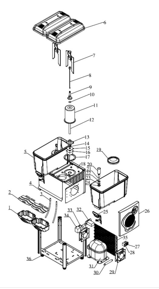
Exploded diagram and spare parts list (CF761)
