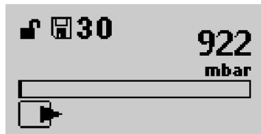
Fig. 11: Evacuation status display (047)
