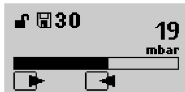
Fig. 25: Gas flushing status display (049)
